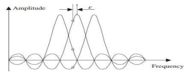
Fig 2: Inter-carrier interference (ICI) subject to CFO.
