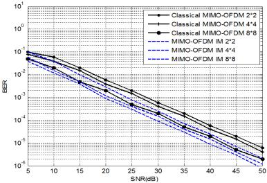
Fig 6: Performance comparison of MIMO OFDM & MIMO OFDM IM using frequency offset for QAM Modulation, MMSE detection.
