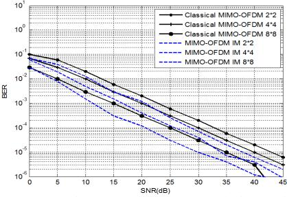
Fig5: Performance comparison of MIMO OFDM & MIMO OFDM IM using frequency offset for QPSK Modulation, MMSE detection.
