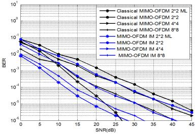
Fig4: Performance comparison of MIMO OFDM & MIMO OFDM IM using frequency offset for BPSK Modulation, ML/MMSE detection.
